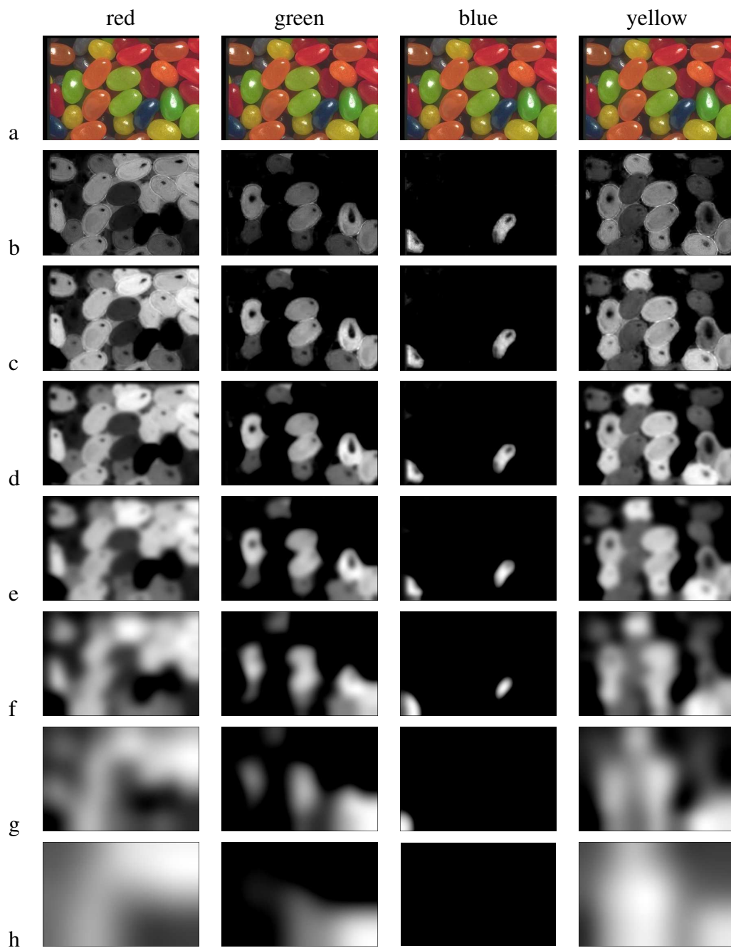
Figure 3.3: From the (a) original image the (b) red, green, blue, and yellow colour channels are created. The first six Gaussian pyramid levels (c-h) are shown. Images originate from the visual attention software.
